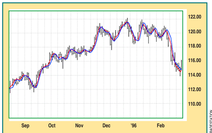
FIGURE 12: IIR AND FIR DATA SMOOTHERS. Note both provide nearly identical responses.
